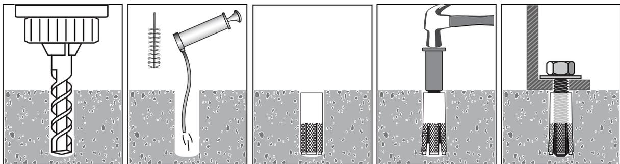
1. Drill recommended hole size, to at least the anchor length in depth.
