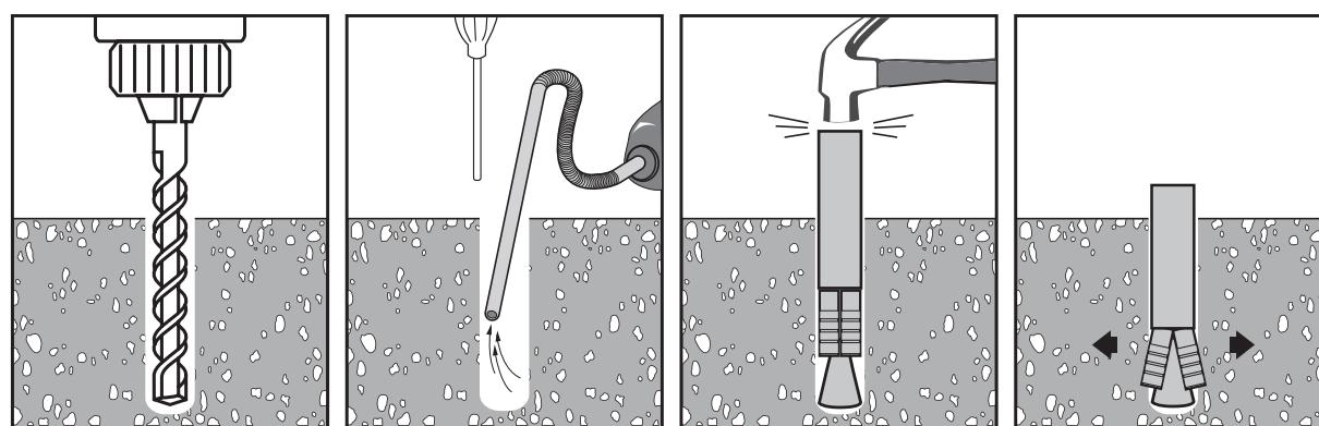
1. Drill hole same diameter as the WD Anchor to the recommended depth.
